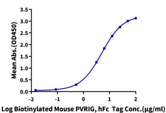
Immobilized Mouse Nectin-2, His Tag at  $2\mu g/ml$  ( $100\mu l/well$ ) on the plate. Dose response curve for Biotinylated Mouse PVRIG, hFc Tag with the EC50 of  $5.04\mu g/ml$  determined by ELISA (QC Test).
